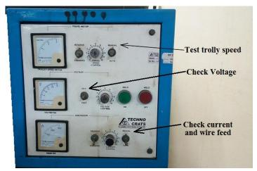
1.6.4 Turn on the power and check travel and wire feed as well as mark the welding line.
